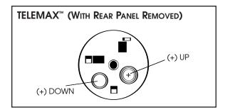
The TELEMAX's two Type 13 (BAT 028) batteries provide up to 150 hours of use, lasting up to six months on standby. Replacement batteries can be purchased from Williams Sound or your local hearing aid dispenser. Your dispenser can also install the batteries.
