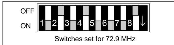
FIGURE 6: SETTING THE T17 FREQUENCY SELECTOR SWITCHES
