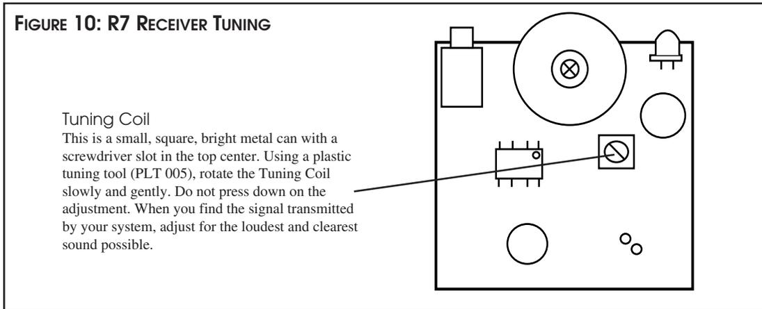
Tuning for the R7 and R-16 Receivers is determined by a single tuning coil. (See Figure 10.) A plastic tuning wrench (PLT 005) is needed to adjust the receiver tuning coil.
