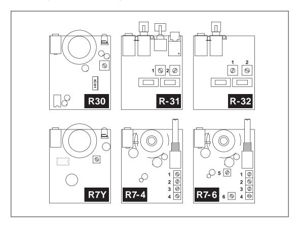
Most Williams Sound single channel Receivers are set at the factory to 72.9 MHz. The standard four-channel receivers (R7-4NA), Channels 1-4, are usually set to frequencies 72.1, 72.5, 72.9, 75.7 MHz respectively. The standard six-channel receivers (R7-6N), channels 1-6, are set to frequencies 72.1, 72.5, 72.9, 75.7, 74.7 and 75.3 MHz respectively.
