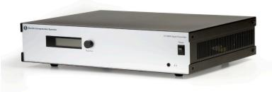
The Digital Transmitter receives the audio input signals and modulates the digital signal. All system settings such as number of channels, channel quality and modulation frequency between 2 and 8 MHz are set on an LCD menu. There are six (6) BNC outputs to lead the signal to the radiators with RG59 cable.
